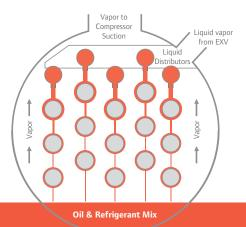
Our patented evaporator design gives the Trane RTWS higher efficiencies using less refrigerant charge, both of which contribute to LEED certification. Refrigerant (red) is uniformly distributed over the first row of tubes. It then flows around them, precisely at the points where heat transfer occurs, to more efficiently cool the fluid (blue) inside.
